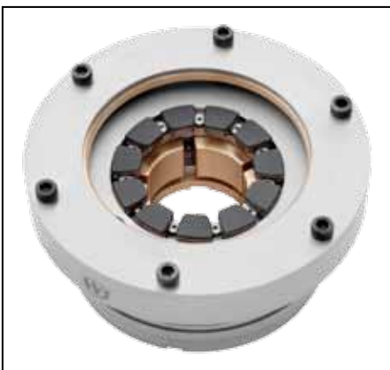
Polymer-lined thrust pads fitted to active face of a combined axial/radial assembly for a 28,000 rev/min heat recovery turbine.
