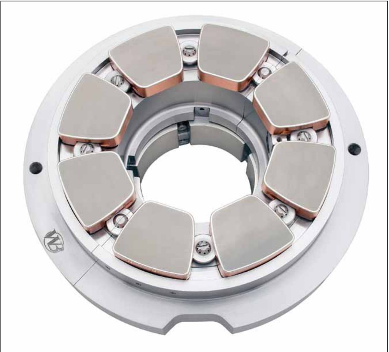
Series 8 main thrust face with copper-chrome pads used in power turbine stage of an industrial gas turbine running at 7,700 rev/min.
