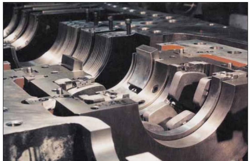
Series 8 Directed Lubrication double thrust bearing in a combined axial/radial assembly fitted to an industrial steam turbine.
