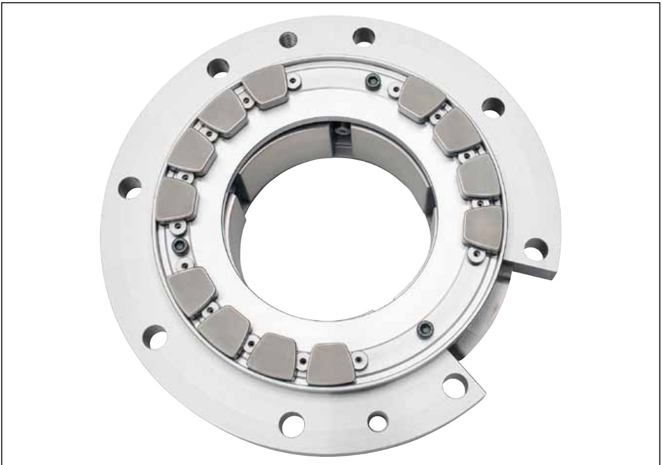
Series 18 Directed Lubrication thrust bearing for use in an industrial gas turbine running at 10,000 rev/min. To reduce power loss, 6 pads were removed on the inactive face of the combined axial/radial bearing assembly.
